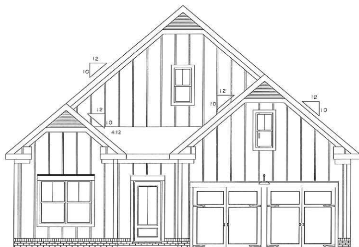
SOMERSET - FRONT ELEVATION "A" - (Brick w/ Board & Batten Siding)
