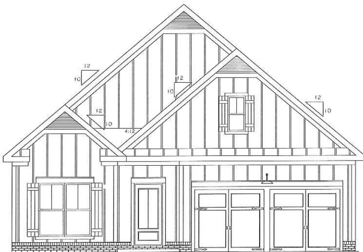
SOMERSET - FRONT ELEVATION "B" - (Brick w/ Board & Batten Siding)
