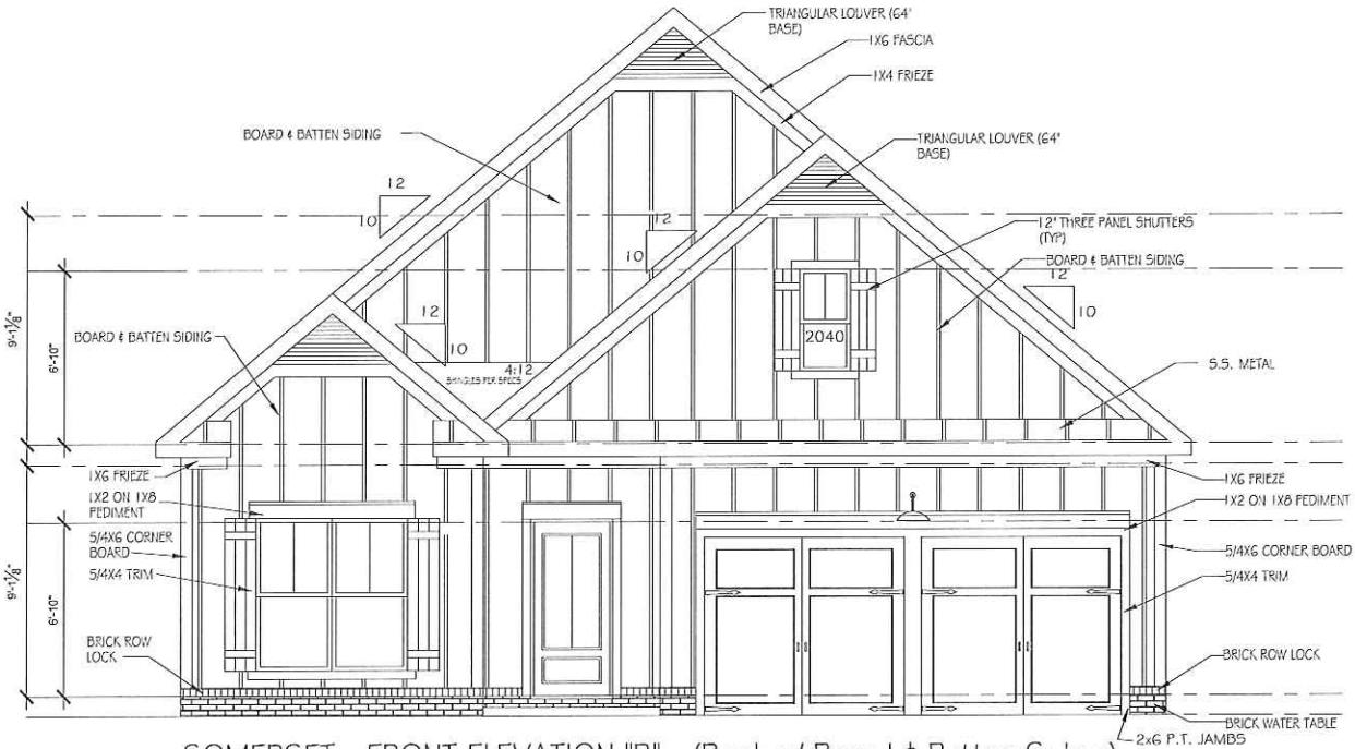
SOMERSET - FRONT ELEVATION "B" - (Brick w/ Board & Batten Siding)
