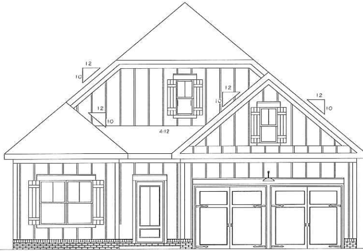
SOMERSET-FRONT ELEVATION "C" - (Brick w/ board & Batten Siding)
